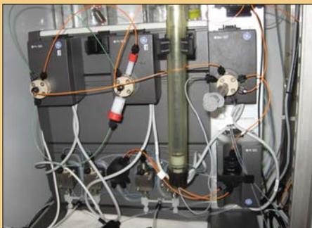
*Hardcore biochemistry: The liquid chromatography apparatus that allows Zhong to fractionate cellular extracts into individual proteins.*
